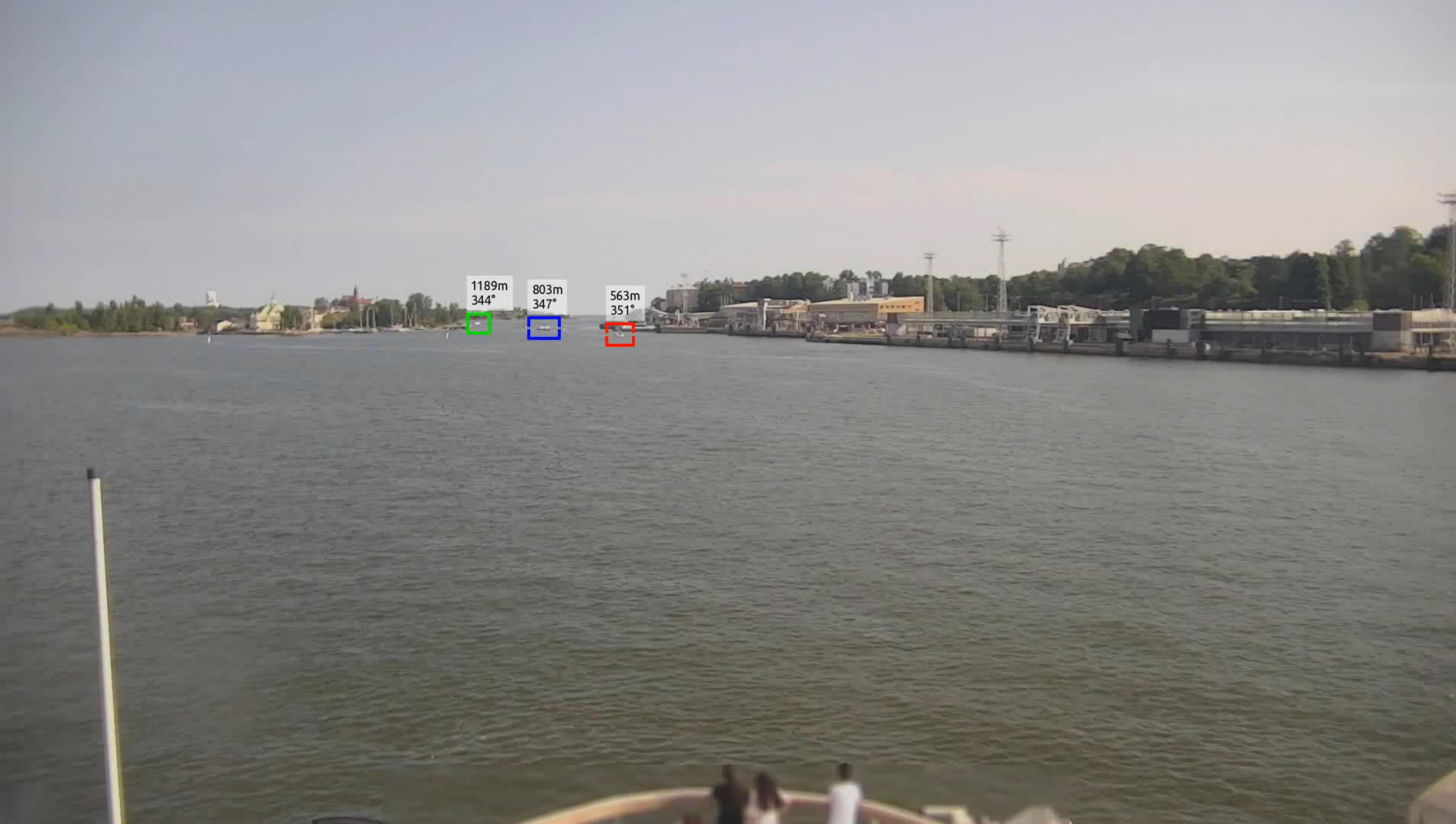
Non-ego vessels' courses and speeds from monocular camera (structure from motion)
