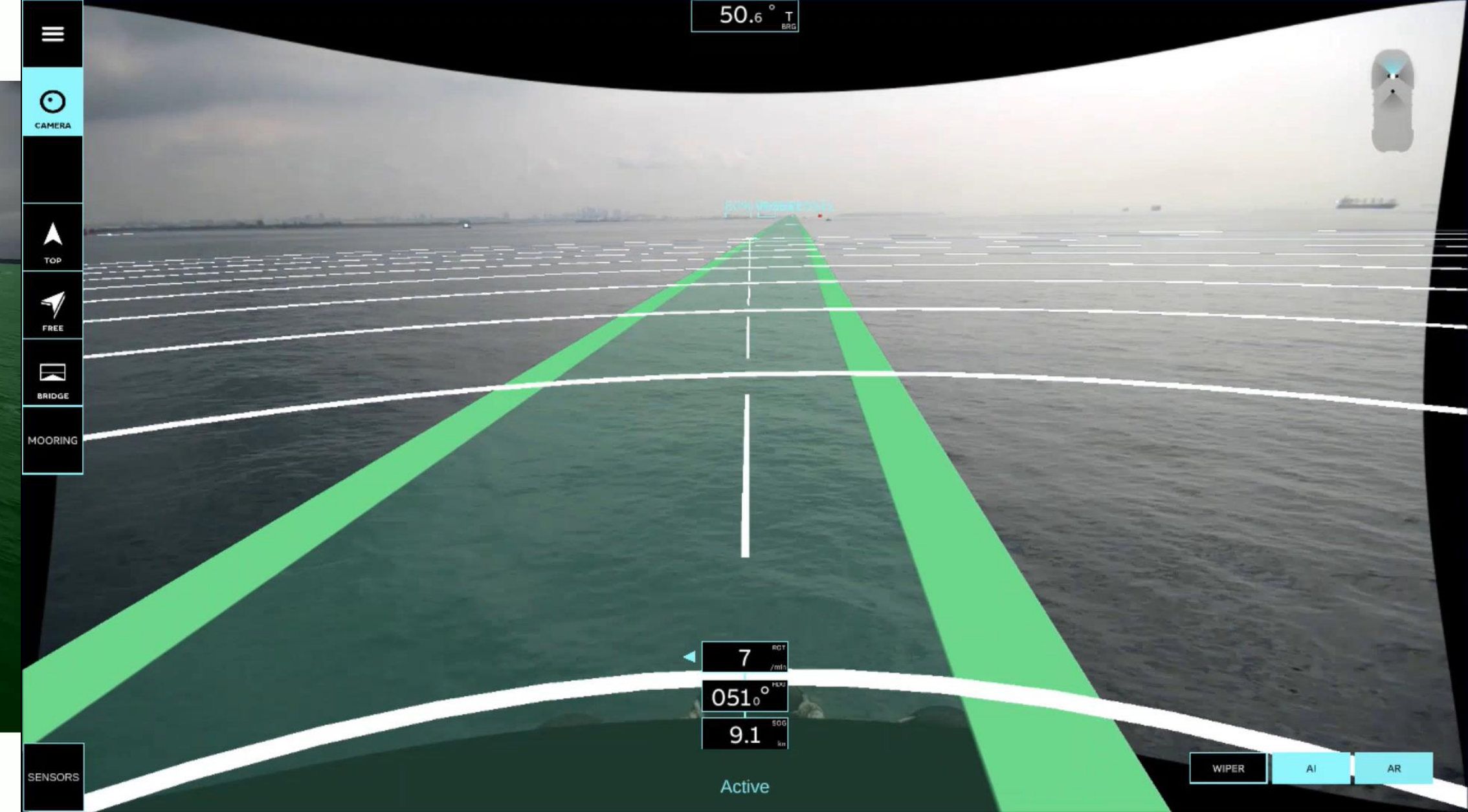
Autonomous collision avoidance of erratically manoeuvring non-ego vessel
